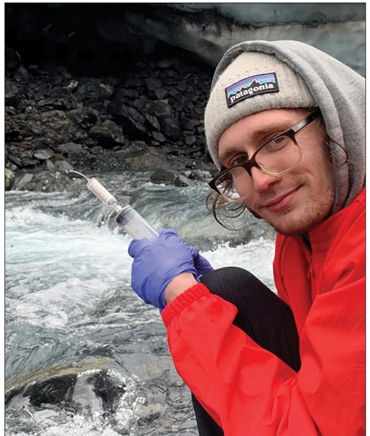
Tyler Fox collecting microbial samples using a 0.22 um filter.
